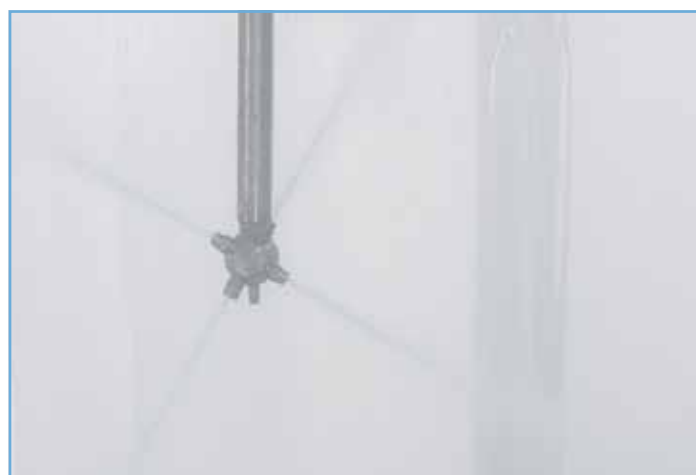
Hydrokinetic head in operation
