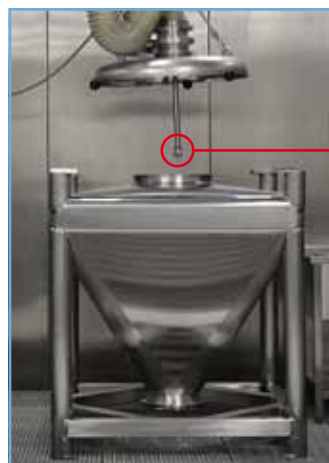
Bin washing/drying station
